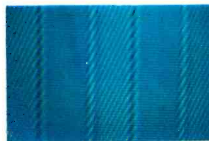
Fig. 9 With the chroma control turned down all the way, only luminance information is visible.
